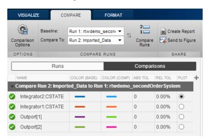
The output from the executed code is within a reasonable tolerance of the simulation data output previously collected in "Generate C Code for a Model" on page 2-2.
